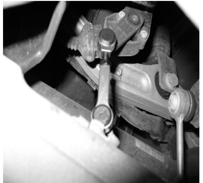
Adjustable Link installed
