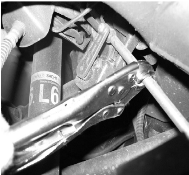
Rear Stock Link removal
