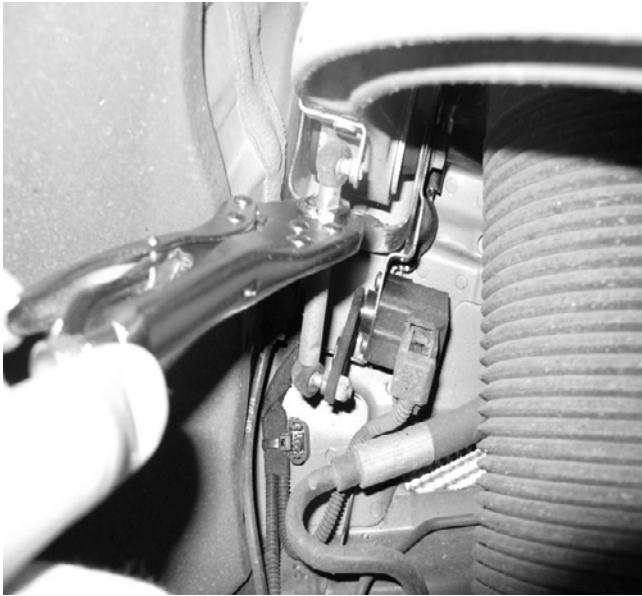
Front Stock Link removal
