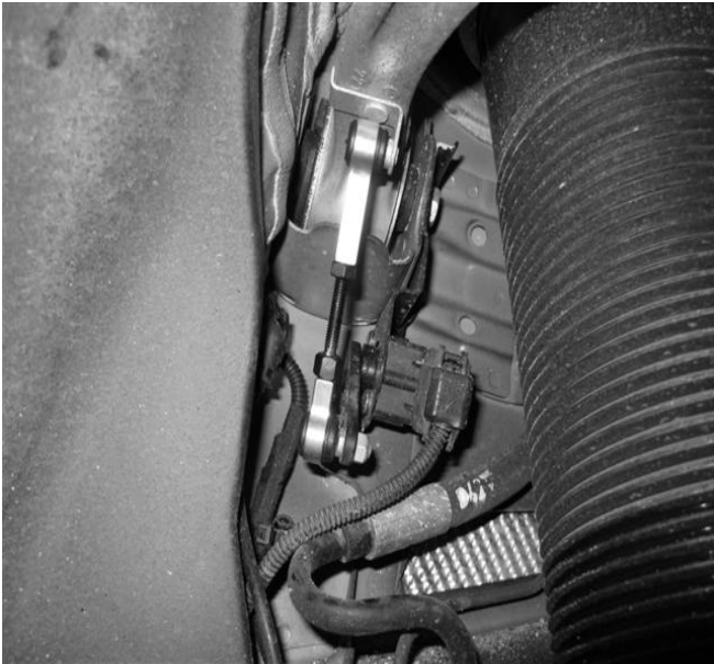
Adjustable Link installed
