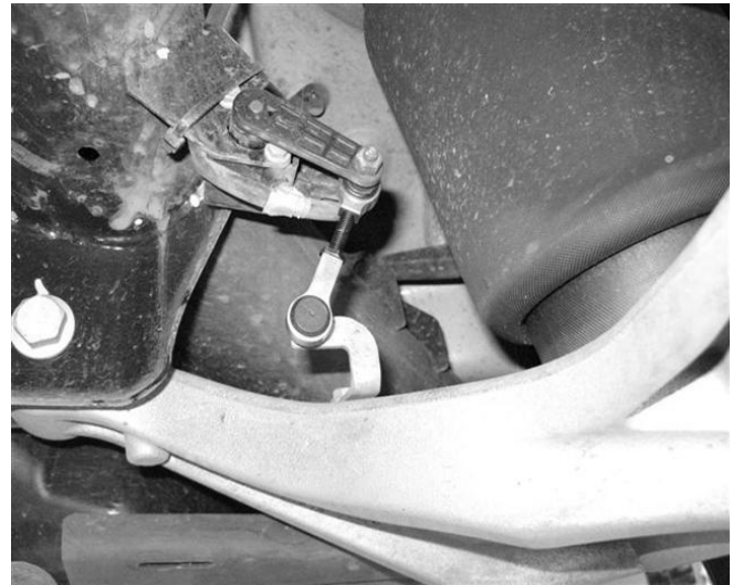
Rear Adjustable Link Installed
