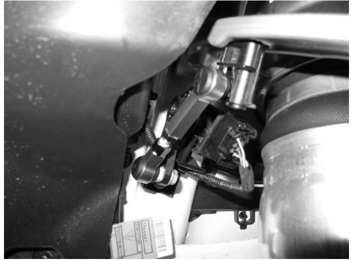
Adjustable Link installed
