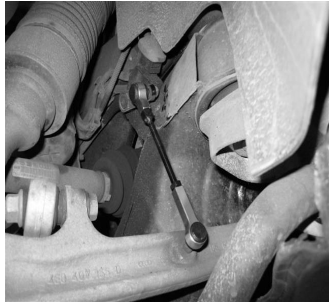
Adjustable Link installed
