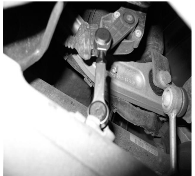
Adjustable Link installed
