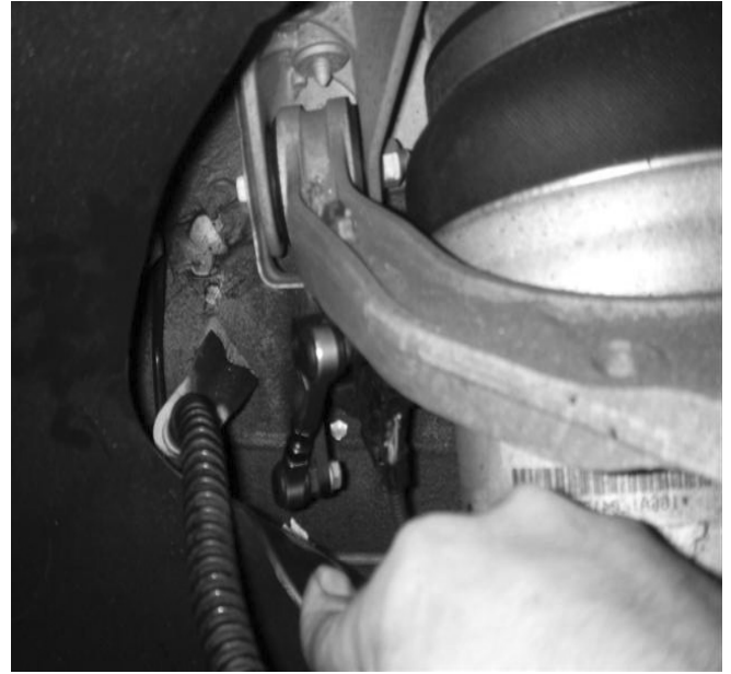
Adjustable Link installed
