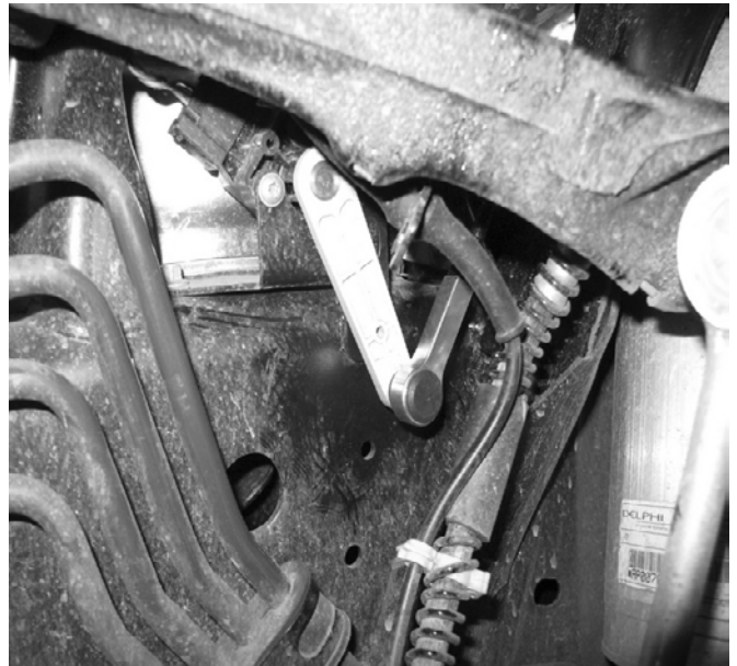
Adjustable Link installed
