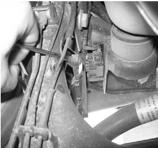
Rear Stock Link removal
