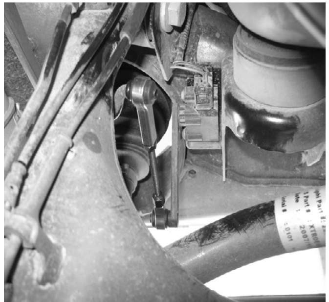
Adjustable Link installed
