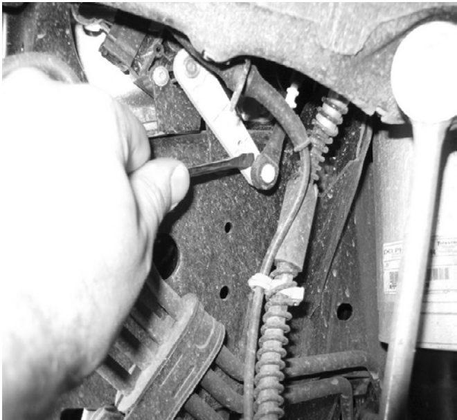
Front Stock Link removal
